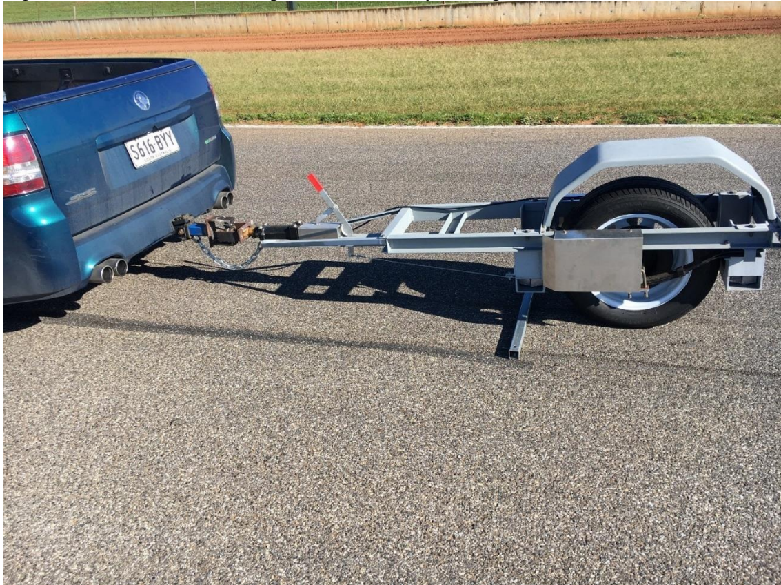
Figure 7 – The on-road tire impact and durability test rig (PSR/LVR version)
