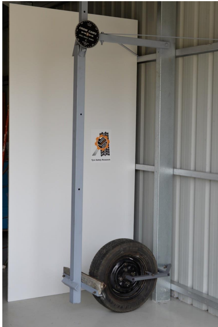
Figure 6 – Simple impact pendulum, dimensionally equivalent to an SAE J1981 impact machine
