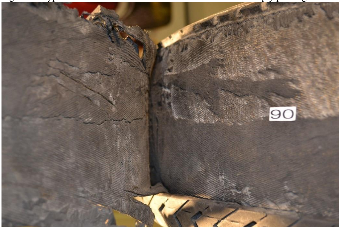
Figure 2 - Typical tread and belt detachment of a steel belted radial ply passenger car tire [6]
