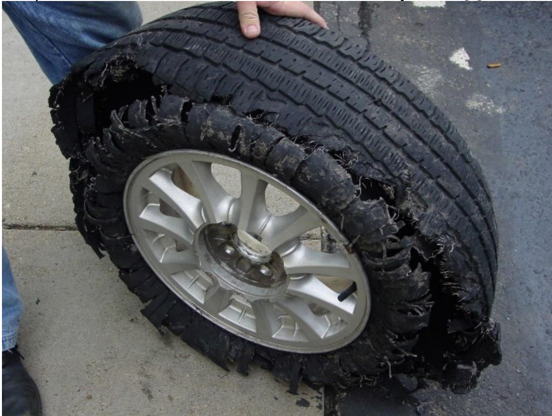
Figure 1 - Tire damage caused by grossly underinflated operation. The sidewalls exhibit multiple fractures, and the shoulders have been circumferentially severed [4].
